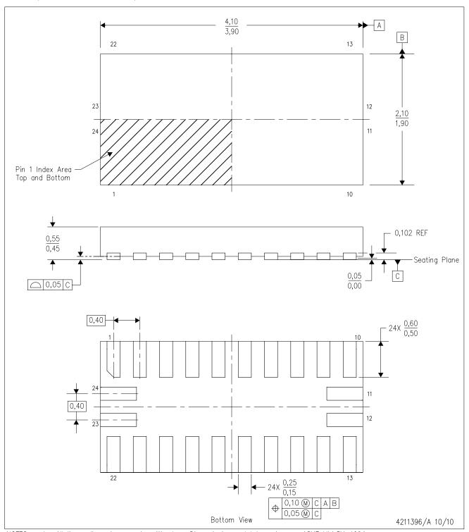
NOTES: A. All linear dimensions are in millimeters. Dimensioning and tolerancing per ASME Y14.5M—1994.
