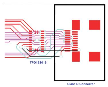
Figure 5. Board Layout for RKT Package
