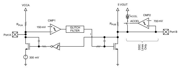
Figure 3. DDC/CEC Level Shifter Block Diagram
